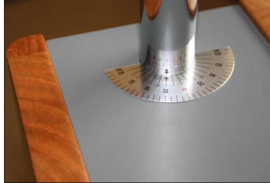
Figure 7: Setting aid angle scale
