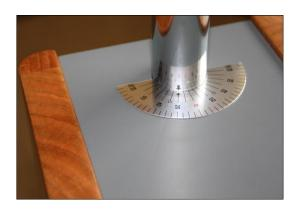
Figure 7: Setting aid angle scale
